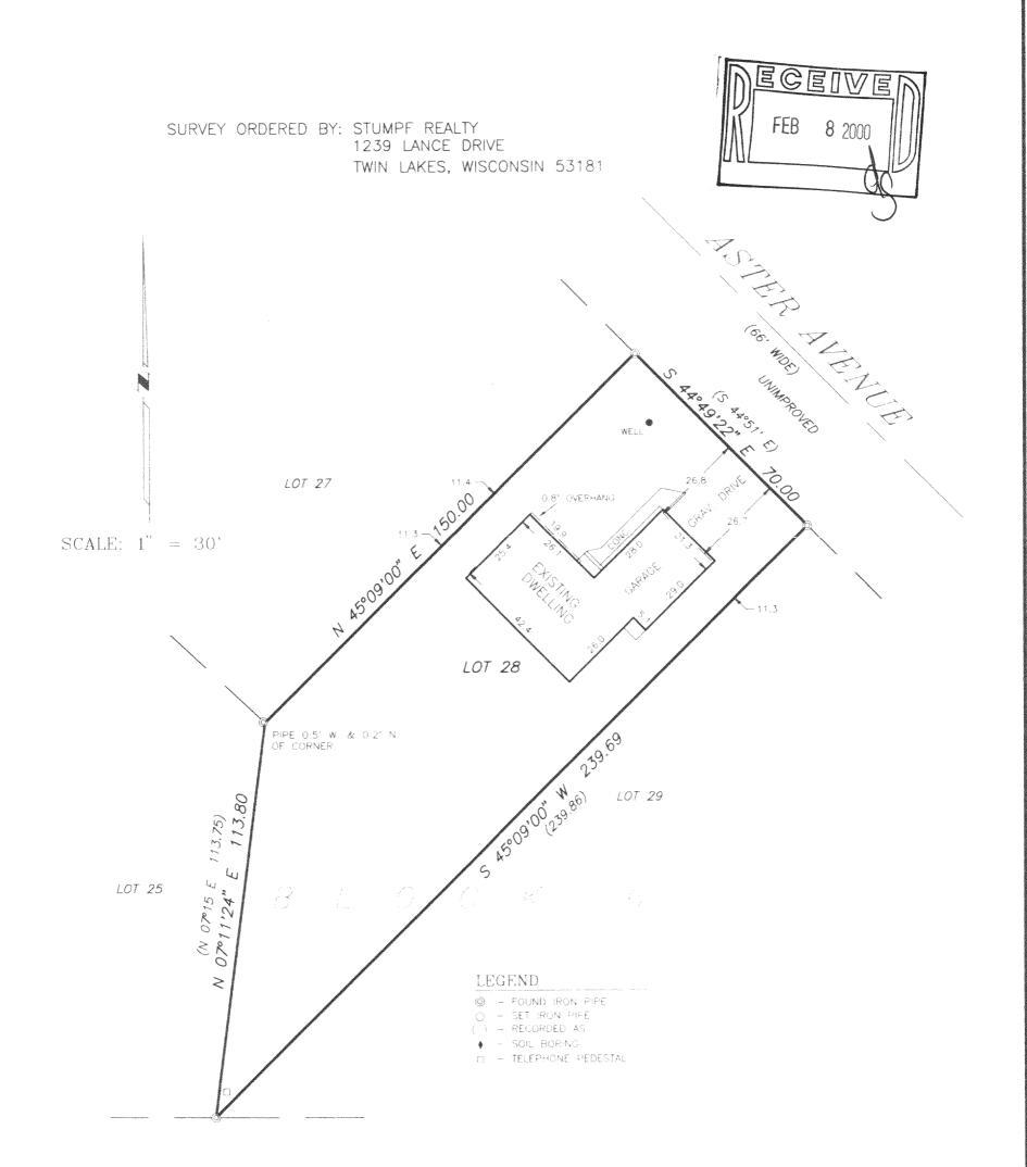
I HEREBY CERTIFY THAT I HAVE SURVEYED THE ABOVE DESCRIBED PROPERTY AND THE ABOVE MAP IS A TRUE REPRESENTATION THEREOF AND SHOWS THE SIZE AND LOCATION OF THE PROPERTY, THE LOCATION OF ALL VISIBLE STRUCTURES AND DIMENSIONS OF ALL PRINCIPAL BUILDINGS THEREON, BOUNDARY FENCES, APPARENT EASEMENTS, ROADWAY AND VISIBLE ENCROACHMENTS IF ANY.
